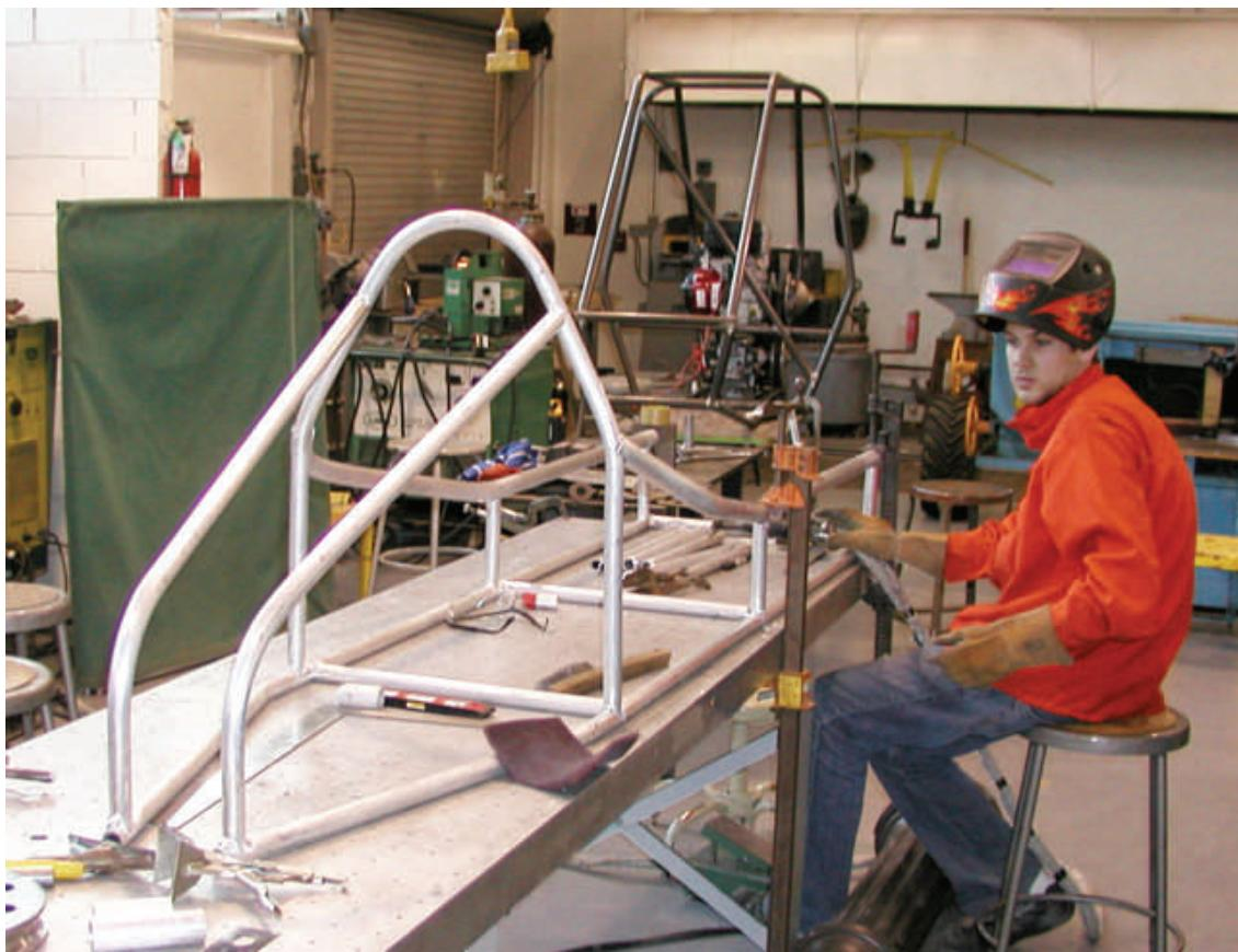
Cutting the Aluminum tubing to length with the appropriate “fish mouth” joint angles, squaring and welding the frame took considerable time.
