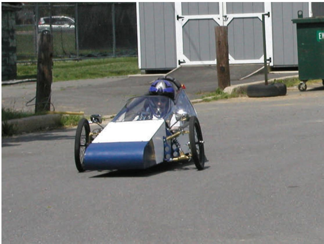
With only a minor tuning of the motor controller (a change in the ramp rate for acceleration), all of the electrical and mechanical systems were working perfectly. Obviously there was time out to paint the car and apply the vinyl lettering.
