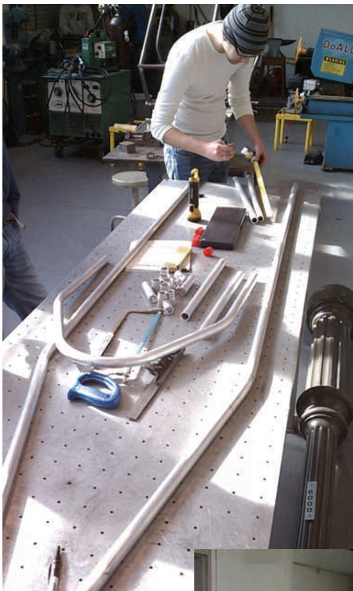
With the frame members verified by the mock-up, Zach began cutting and forming the aluminum tube on the assembly table. The basic frame material size was 1 inch OD, while the side impact members were 1-1/4 inch OD tubing.
