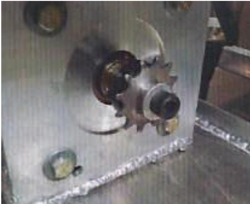
An adaptor was machined to mount a 12 tooth sprocket faced down to accept an ANSI standard #40 bicycle chain. The sprocket is mounted rigidly to the motor shaft.
