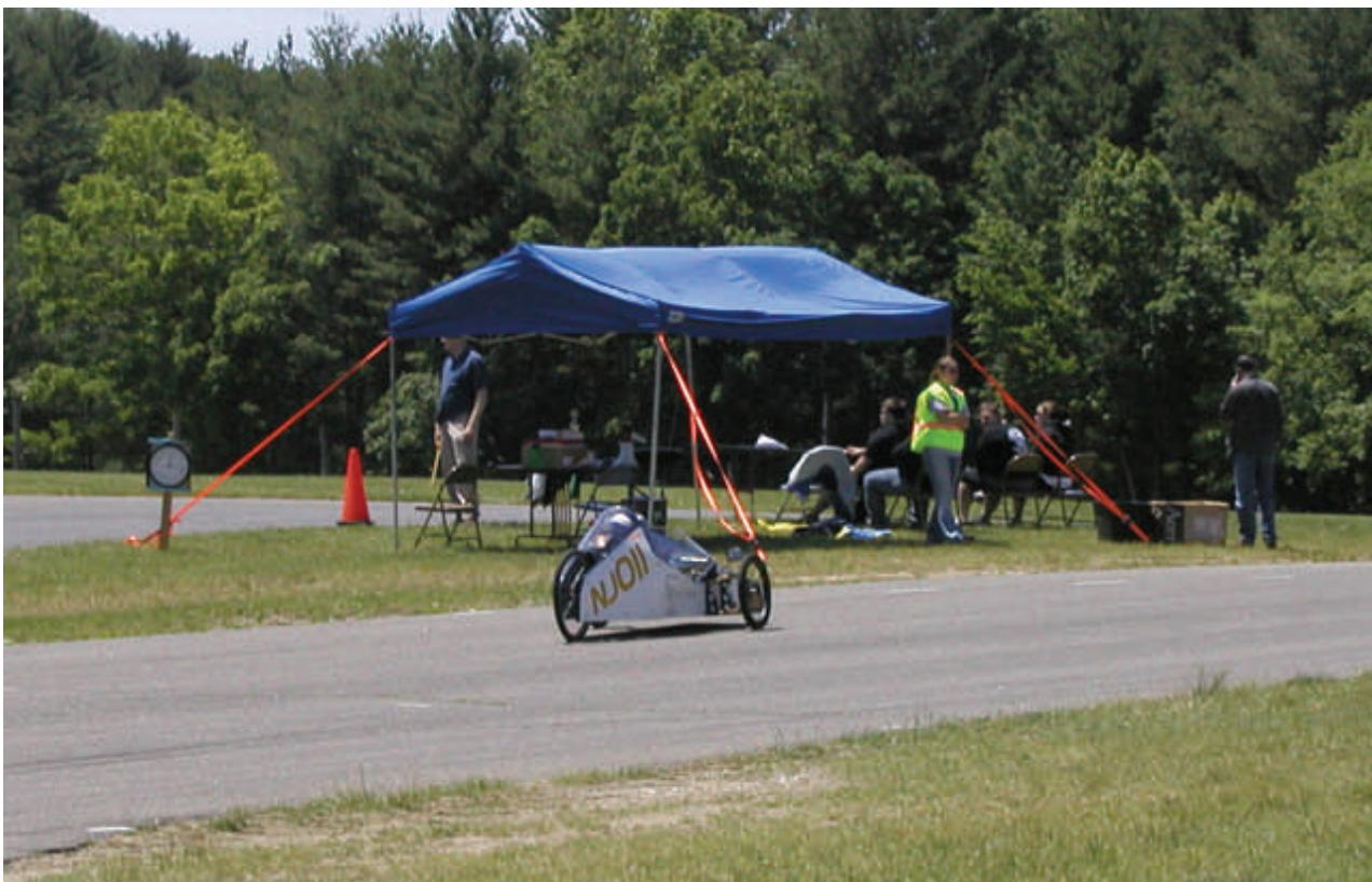
Into the pits following the spin, the car had to be inspected and a driver change had to be accomplished. The rear wheel was found to no longer be true. We could continue to run at the same speed as the leading cars, but a high speed finish was out of the question.
