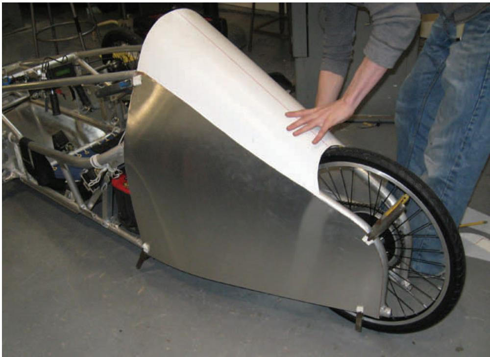
The Lexan polycarbonate cover (shown above with it's protective cover) is held in place in preparation for locating dzus fasteners for the rear side covers. The polycarbonate material was chosen for this rear cover area to insure that no interference would be created for the telemetry box mounted high in this area.
