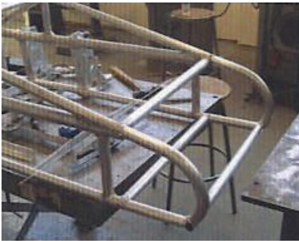
A change was made to the nose section. Hunter, being the taller of our two drivers, needed more room for his feet. We also needed an area to mount the peak power tracker for the solar array. Both were accommodated by extending and bending the roll cage tubes and welding them to extended bottom tubes.
